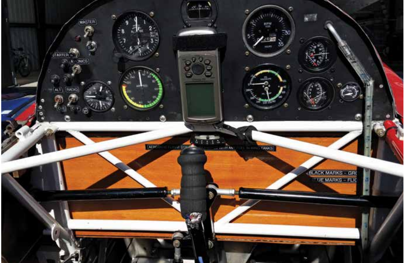
The black stripes that can be seen in the top and bottom of the hefty solid wood main spar are carbon fiber layers, responsible for providing a virtually unlimited wing loading capacity with nearly zero flex.
